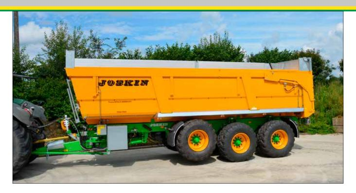
JOSKIN offers now hydraulic, adjustable and practical extensions for the Trans-SPACE 7000/125 and 8000/150 agricultural trailers. They make the loading operations easier and allow the total transport volume to be increased. The extra DIN volume is of  $8.4 \, \text{m}^3$  on 7000/125 and  $9.4 \, \text{m}^3$  on 8000/150.
